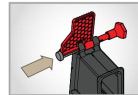
**STEP 4.** Insert pivot pin as shown, then remove large PPT pin. Finally, remove PPT fixture and snap pivot pin into closed position.
