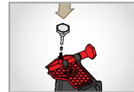
**STEP 2.** Load spring first, then detent second into the PPT fixture. Compress the spring and detent with the PPT plunger and hold.
